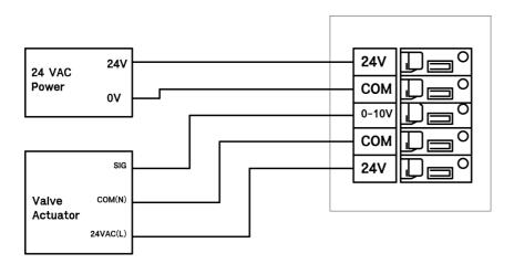
AC24V and AC 24V, GND and GND - inside PCB common
